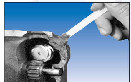
RK 454 Repairs Cast Iron Housing
