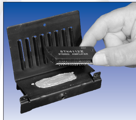
Duralco™ 132 Dissipates Heat in a Semiconductor Device
