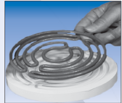
Placing Heater Coils in Insulating Disk
