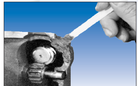
RK 454 Repairs Cast Iron Housing
