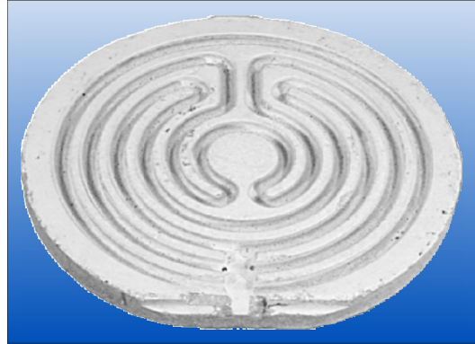
Mold for making a Heating Coil Insulator
