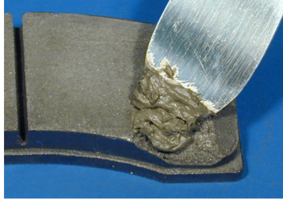
7032 Repairs a Wear Plate
