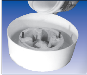
Pouring Replicast Around a Model
