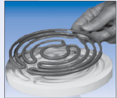
Placing Heater Coils in Insulating Disk
