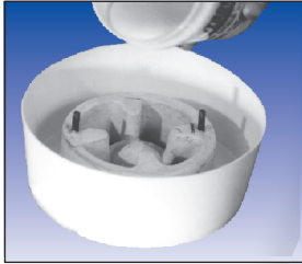
Pouring Replicast Around a Model
